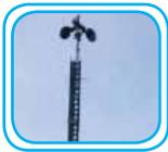
A built in anemometer evaluates the wind potential. Within some months (based on the wind measurement results) we decide if the wind potential of the area is sufficient for the installation of a wind turbine.
